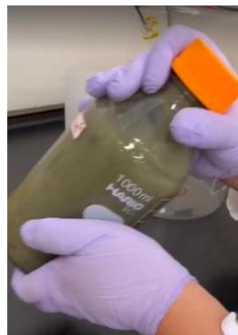
Stir adsorbent with wastewater
