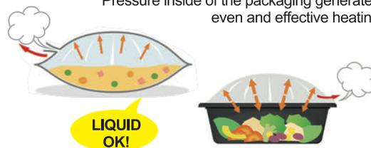
The steam vent located on upper part of the packaging prevents from liquid leaking.
