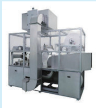
2. Apparatus for forming a sheet of nanofiber
